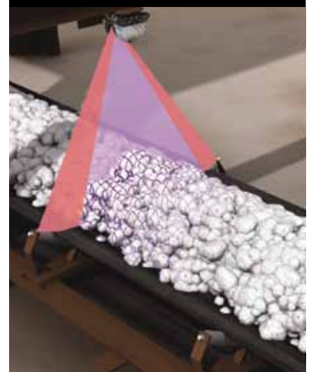
Figure 7: bulk edge and conveyor edge monitoring
